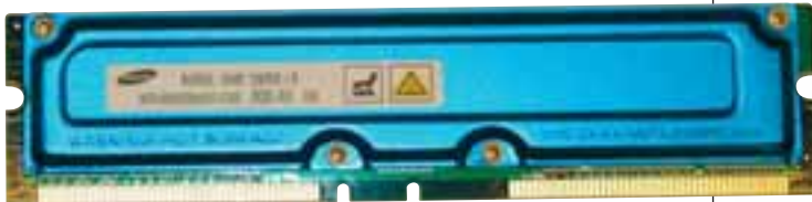
Rambus Rimm modules were used in some early Pentium 4 PCs
